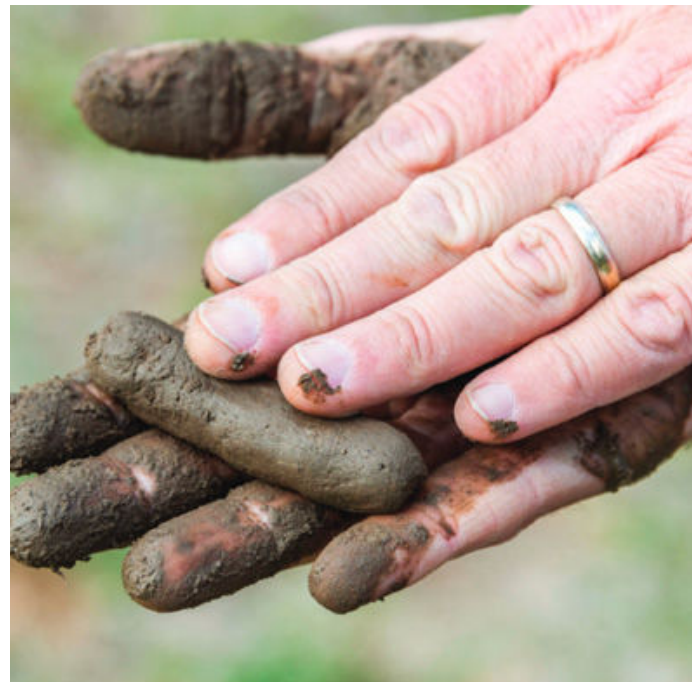
A ribbon test to determine soil texture
