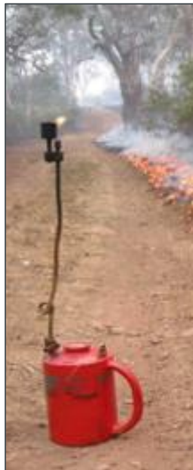
Figure 31 – A drip torch is a useful tool to assist with lighting a burn. Correct ratio is 3 parts diesel to 1 part petrol.
