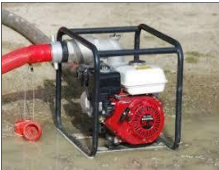
Figure 34 – Fire pumps are very useful to draw and pump water from a range of water sources.
