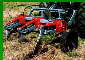
Yeoman's plow and Agrowplow, showing coulter discs and aerator shanks
