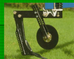
Yeoman's plow and Agrowplow, showing coulter discs and aerator shanks
